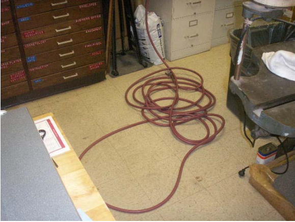
06-6 The cord in the print shop should be coiled and stored off the floor. This should reduce the potential for injury due to tripping.
