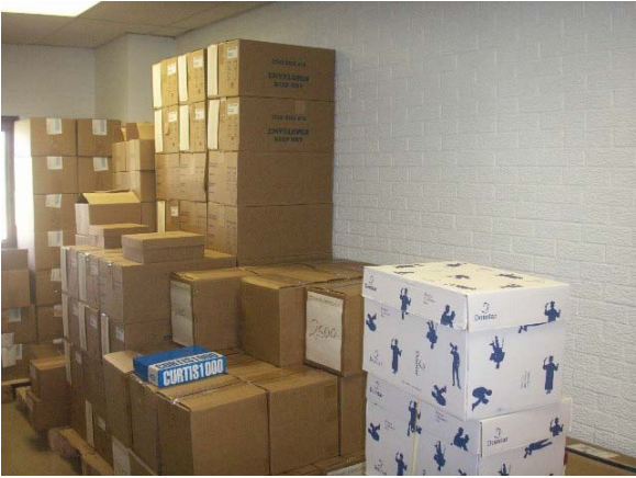
06-7 The storage in the printing room should be reviewed. The height of the storage may make it unstable and pose a hazard while trying to retrieve the upper most items. Limiting the height may reduce the potential of injury.
