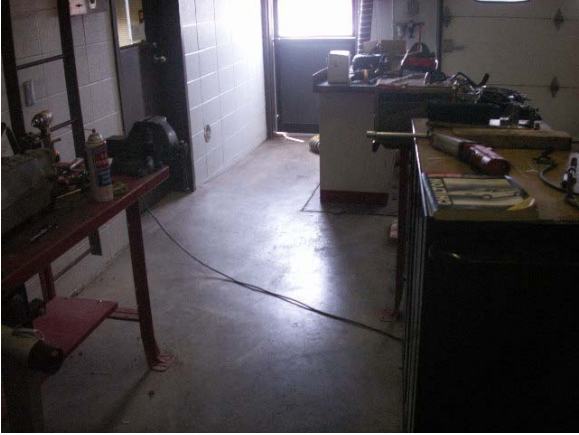
06-3 The cord should be relocated. If this is not possible it should be covered with a cord cover. This should reduce the potential for injury due to tripping.
