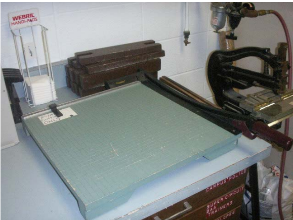
06-5 Finger guards should be installed on all paper cutters. This should reduce the potential for injury due to employees getting their fingertips under the cutting blade.
